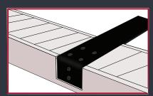
The CounterPlate Plus is designed to attach to half walls or pony walls, supporting overhangs on "breakfast bar" style countertops. This "L" shaped bracket ties in to the vertical wall studs for improved strength and stability.
