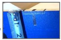
Using a circular saw, or oscillating multitool, cut out the marked area and test fit the bracket as necessary.
